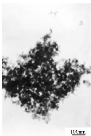
FIG. 3. The TEM image of the pure hexagonal phase Cu 2-x Te nanocrystallites.
